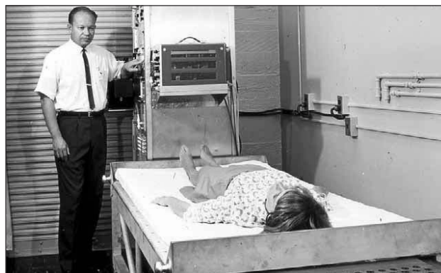
Hal Anger in 1965 with the whole-body scintillation scanner at the Donner Laboratory. The small holes in the foreground are part of the collimator. From the collection of Henry N. Wagner, Jr., MD.
